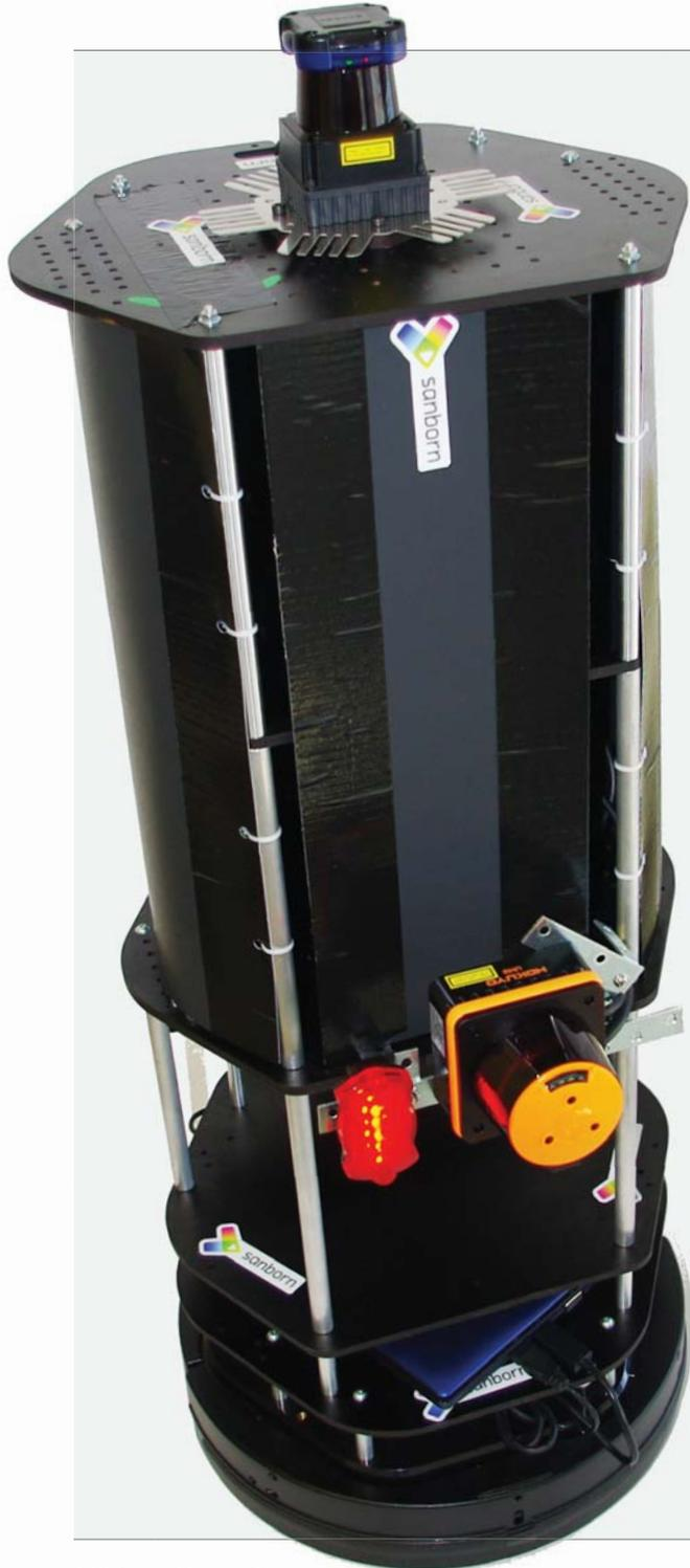
**Safety**—Collection at speeds slower than average human walking speeds and real time detection of obstacles (humans and environment features) while maintaining a Class 1 Eye Safety Rating makes it safe for indoor environments. Human joystick override available for emergency situations.
